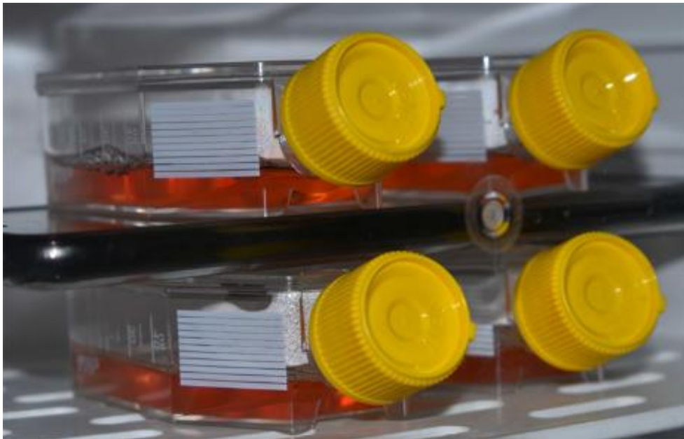
Figure 1: Experimental setup during exposure with duplicate samples on the mobile phone display (= direction of radiation towards the user) and beneath the mobile phone (= direction of radiation away from the user).
